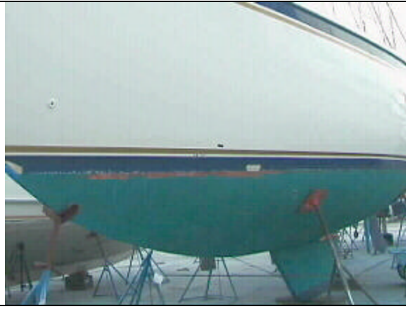
Delamination in the hull of a fiberglass boat.
