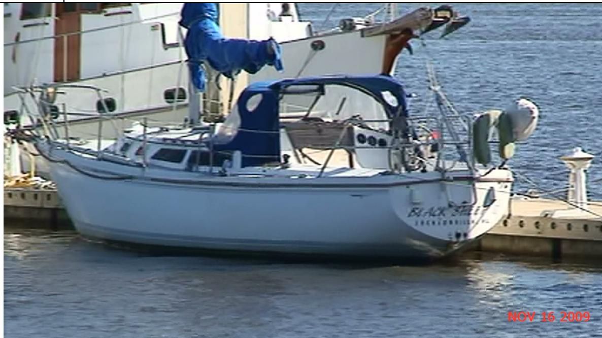
Vessel is tied starboard side to the floating dock. Evident in the photograph is the insert on the rub rail which is coming apart from the bow extending back to the lower aft shroud.
