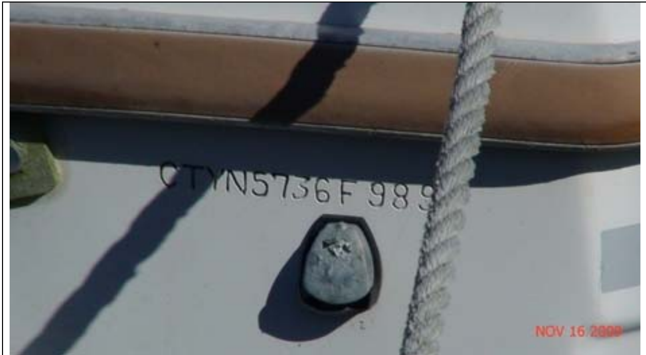
Digital Photograph of HIN Note that this was engraved into the hull rather than imprinted from the mold.
