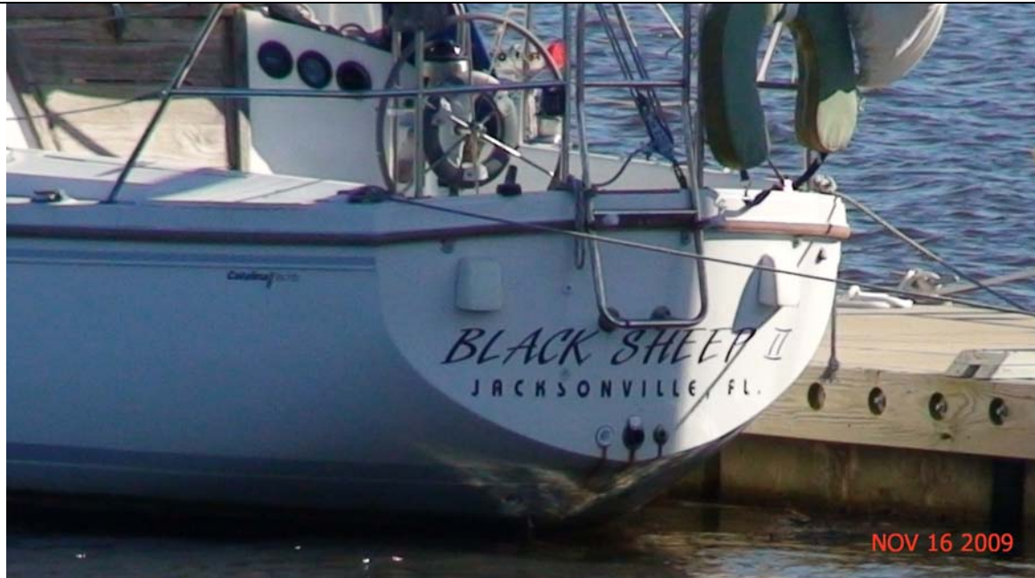
Stern view showing Vessel Name and Hailing Port. Evident are the TYPE IV PFD, portable LPG grill, steering with autopilot, forced ventilation cowls, boarding ladder cockpit drains and engine wet exhaust port.
