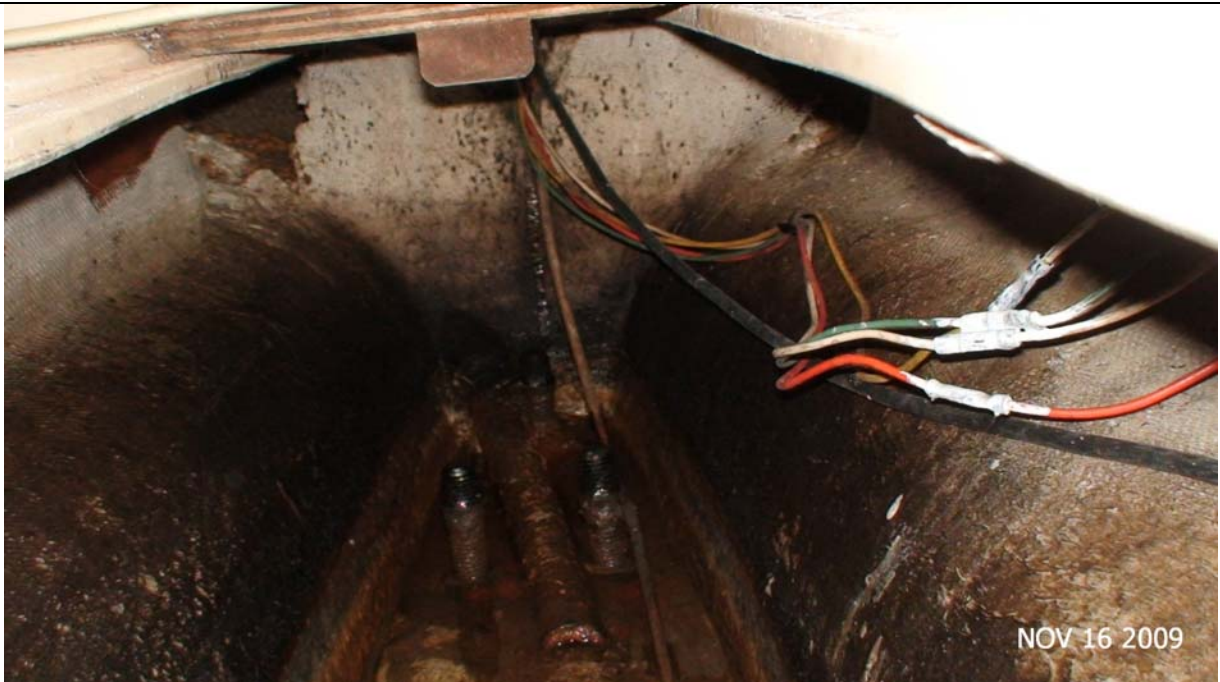
Keel bolts need to be cleaned and treated, bilge needs to be cleaned, 12vDC wires need to be supported.
