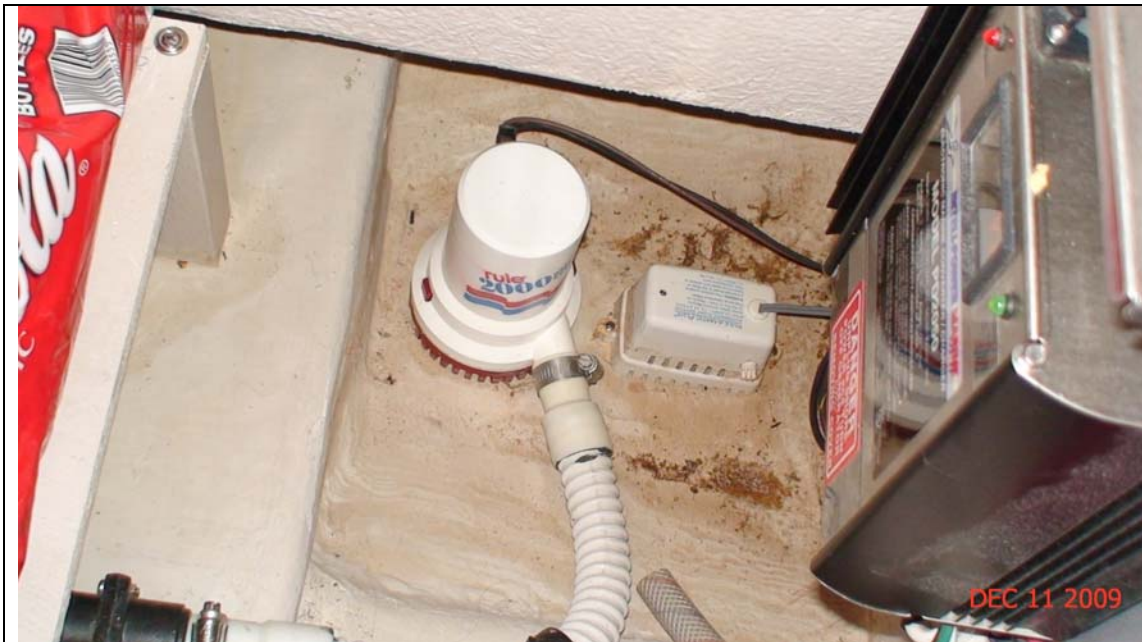
Forward bilge pump. Bilge was dry but had some debris that needs to be cleaned.
