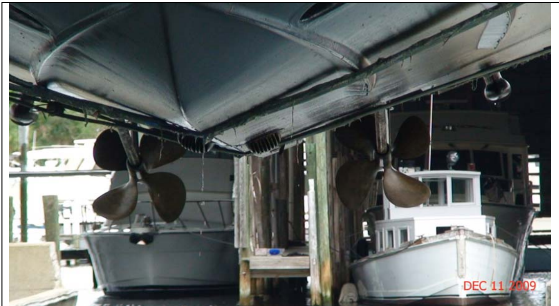
View of underwater running gear when vessel was hauled for bottom inspection.
