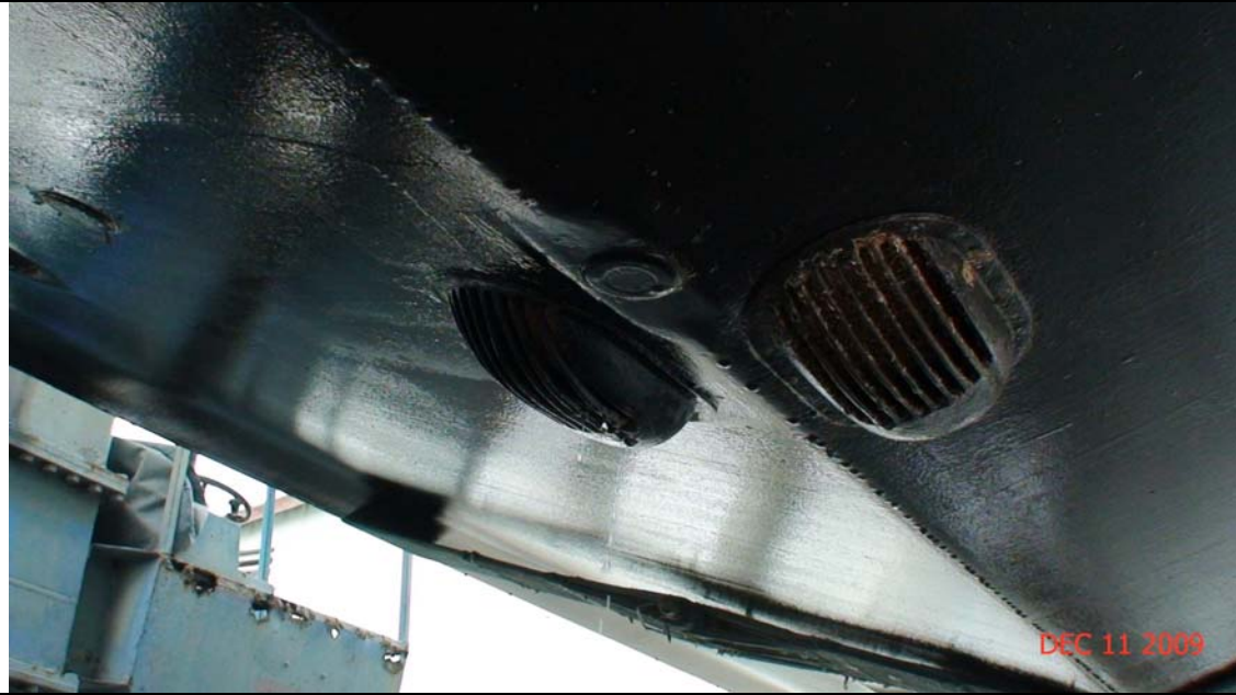
Raw water intakes for CUMMINS engines and transducers for depth meters.
