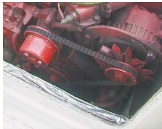
Black dust from the fan belt attached to the alternator. Check belt alignment and renew belt as needed.
