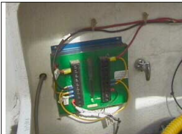
View of Ample Power device used to ensure that engine starting battery is always fully charged.
