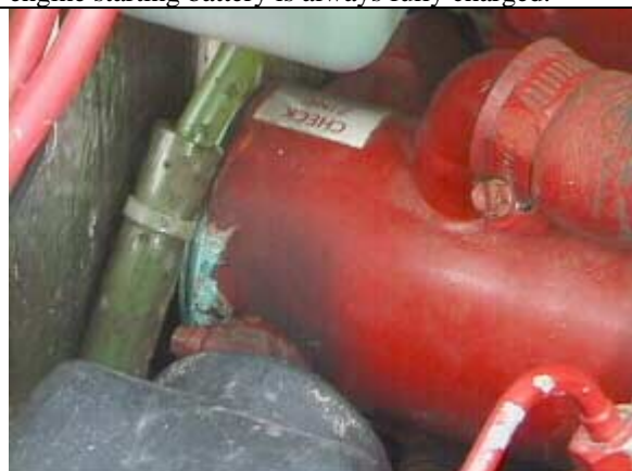
View of turquoise corrosion on heat exchanger. Check the condition of the sacrificial pencil zinc.
