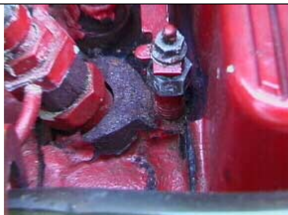
Rust developing on surface of engine and around injector ports. Clean, repaint, and treat with anti corrosion compound.
