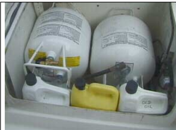
Propane tanks in dedicated propane locker. Locker drains overboard.
