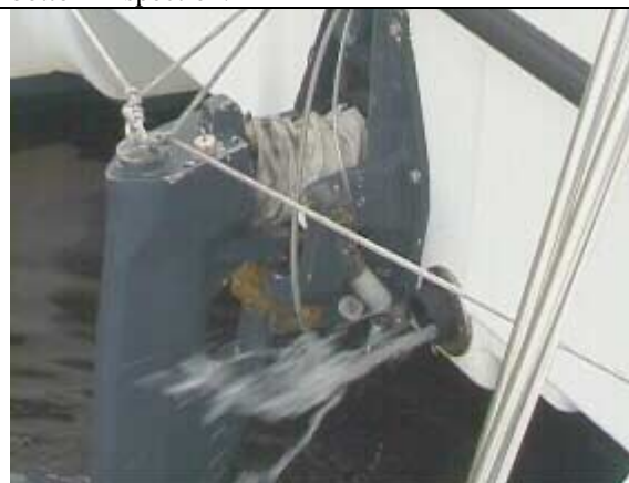
View of the outdrive and the engine exhaust port (lower right hand portion of photograph). Water flow was adequate and engine did not overheat during seatrial stress test.
