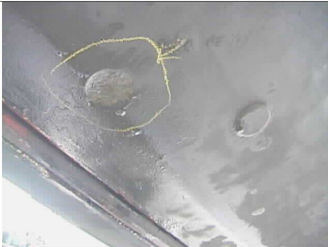
Starboard hull near transducer. The circled area shows where the hull was ground out (3 inches in diameter) and not faired back to the shape of the hull.
